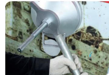
Final tightening with locker lever
