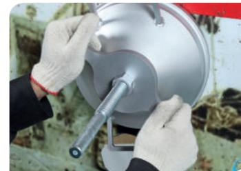
Tighten with lock nut (with locker)
